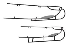
Most fingers will naturally align with the top of the guide. If users with small fingers have difficulty aligning their whorl (gray oval) with the center of the sensor, take extra care to place the center of the whorl in the center of the sensor. For most people, the whorl center is directly opposite the fingernail's cuticle. If in doubt, use the cuticle as a guide.
