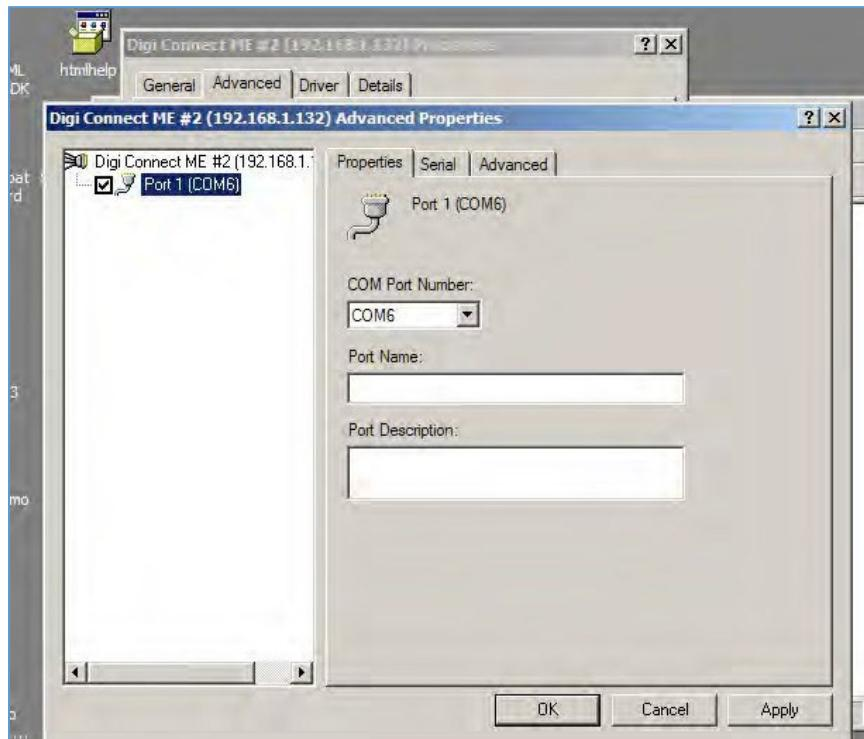
It is important to note though that changing the COM port setting after installation will require that the SigPlus.INI file be altered either manually or through [SigPlus Adjust](#).
