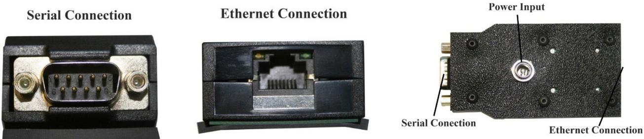
Once the power supply, Topaz pad, and ethernet cable (also connected to the Network Hub) is connected, an orange light (for network connection) and blinking green light (for power) should be visible, denoting the ethernet adapter is functioning.
