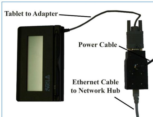
Once the adapter is properly setup, now the user can proceed with the software installation. In order for the ethernet adapter to work properly, users need to install the proper version of SigPlus, (SigPlusE). This version can be downloaded at: <http://www.topazsystems.com/Software/sigplus.exe>.
