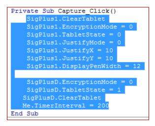
31. Once the code is copied, paste it into the code for the sample table that was created. This will ensure that the proper coding is attached to the "Capture\_Click" event.
