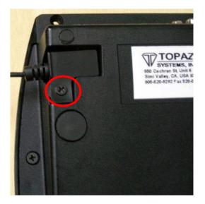
3. Remove the bay cover and remove the 1/8" plug from the Topaz tablet and replace it with a new e-tether pen.
