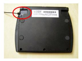
2. Remove the screw that secures the bay cover to the Topaz tablet with a Phillips screwdriver. This cover prevents the pen from being removed from the pad.
