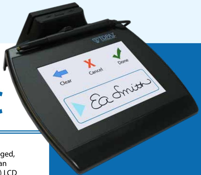
The Topaz SigGem® Color 5.7 MSR is Topaz's largest, rugged, and advanced biometric electronic signature pad with an attached MSR and 5.7 inch, full-color TFT VGA (640x480) LCD that captures and displays "electronic ink" under the pen tip for a natural signature.
