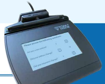
The Topaz<sup>®</sup> SignatureGem<sup>®</sup> LCD 4x3 MSR is Topaz's mediumsized, rugged, advanced electronic signature pad with an attached MSR and transflective LCD that displays "electronic ink" under the pen tip during signing.
