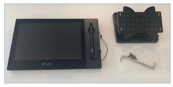
Included with the A-TSL2-1 is the tilt stand, dual-sided screwdriver, and four screws.
