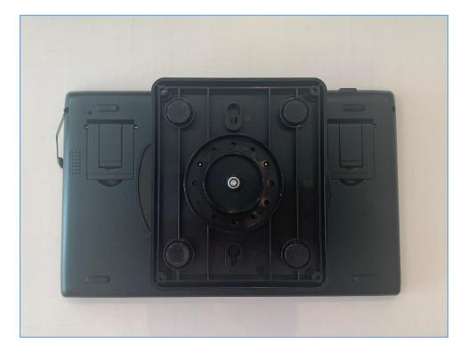
4) Starting on the right side, insert 2 of the screws and tighten using the provided screwdriver.
