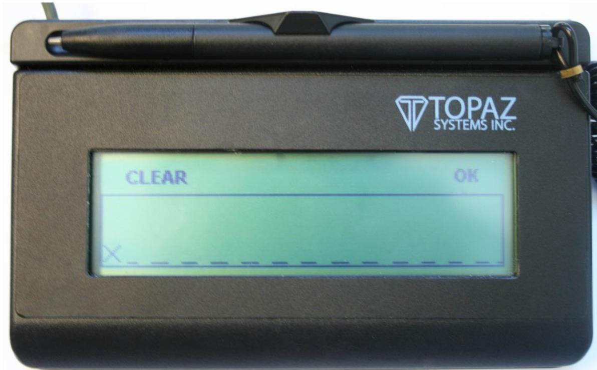
Sign on the dotted line on your tablet, and you will see the signature on the tablet, as well as on the “Topaz LCD 1x5 Demo” on your monitor (as shown below).
