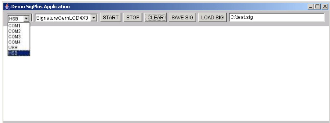
Now, ensure that the “Tablet Model” you are using corresponds to the tablet type selected by the demo application. For the purposes of this demo, we used a SignatureGem LCD 4X3.
