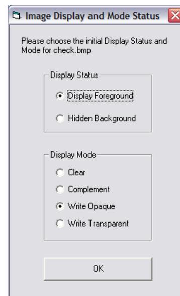
Each image placed will entail a choice of background or foreground placement, as well as the display mode (these will later correspond to the first and second arguments of each use of the LCDWriteBitmap method). These choices will appear in the “Image Display and Mode Status” window. Once the desired choices have been made, simply click “OK” to place the image.
