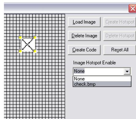
When an image is chosen for "hotspotting", you can drag the hotspot outline directly on the image, and press the "Create Hotspot" button to create a hotspot there. The hotspot will be created behind the image, so if you want to delete it later you will have to move the image out of the way.
