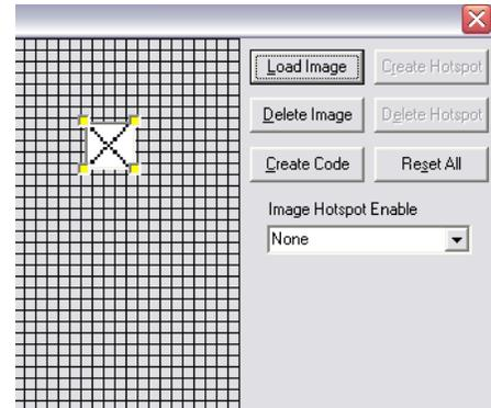
Here is how check.bmp has been loaded into the “Position Window”. Once the image is loaded, simply drag and drop to move it into the desired location. To delete an image from the “Position Window”, right click on it. This will bring up four yellow boxes on the corners of the image signifying that the image has been selected. When an image displays these yellow markers, it cannot be dragged and dropped. Simply click again on the image to get rid of the yellow delete markers.
