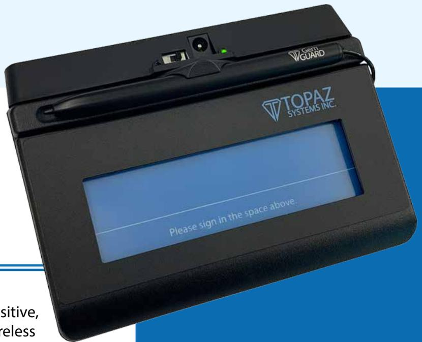
The Topaz® SigLite® 1x5 BT is a small, pressure-sensitive, low-cost electronic signature pad designed for wireless applications using Bluetooth connectivity. It features all the high quality biometric and forensic capture techniques of a SignatureGem® 1x5 signature pad but with a touchpad and stylus in place of the active electromagnetic pen and sensor, making it both space-saving and cost-efficient.
