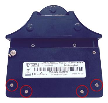
4) Take the four rubber feet and stack one on top of the other to create two stacks of two rubber feet. Then, place them near the bottom of the back of the pad (in between the screws) and press firmly. These will serve as spacers when mounting the pad on the tilt stand.
