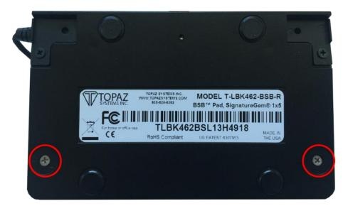
4) Using a small Phillips screwdriver (not included), remove the four screws circled below. Keep the small black screws (circled in blue below) separate from the small silver screws (circled in red below). The small silver screws will be reused in Steps 7 and 8 on Pages 7 and 8.
