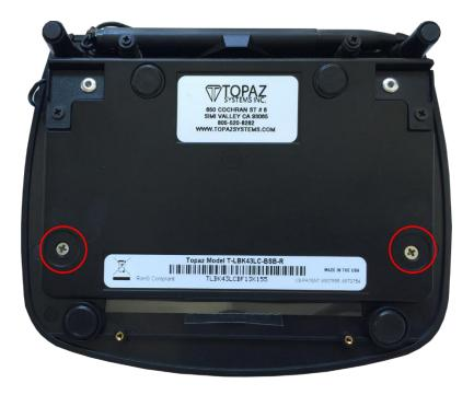
4) Using a small Phillips screwdriver (not included), remove the four screws circled below. Keep the small black screws (circled in blue below) separate from the small silver screws (circled in red below). The small silver screws will be reused in Steps 7 and 8 on Pages 7 and 8.
