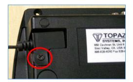
3. Remove the bay cover and 1/8" plug from the Topaz pad; replace it with the new e-tether pen.
