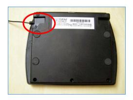
2. Remove the screw that secures the bay cover to the Topaz pad with a Phillips screwdriver. This cover prevents the pen from being removed from the pad.
