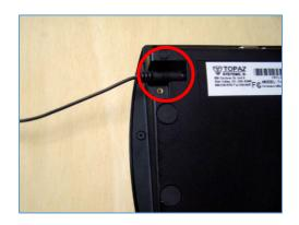
4. After the e-tether pen is replaced, replace the bay cover and screw to secure
